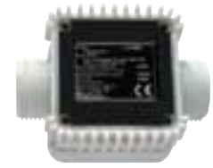
K24 Pulse-meter Flow rate up to 100 l/min Accuracy \pm 1\% Pulse out 100 p/l
