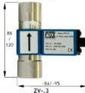
\*ZV\* flow indicator is available in two versions, with an exchange electrical contact or with a proportional 0-10 V output signal. The operating point, in the electro-mechanical version, is reached sliding along the axis of the instrument the connector's saddle and locking it with an M3 screw. In the execution with proportional output the connector is fixed in factory.
